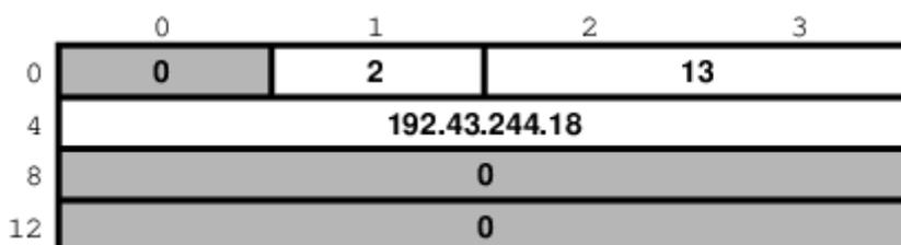
By the way the `sin_addr` field is declared as being of the `struct in_addr` type, which is defined in `netinet/in.h`:
